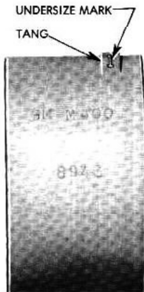
Figure 60-91 - Location of Undersize Mark on Bearing Shell
