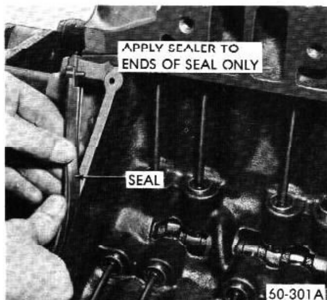
Figure 60-73 - Intake Manifold Seal Installation
