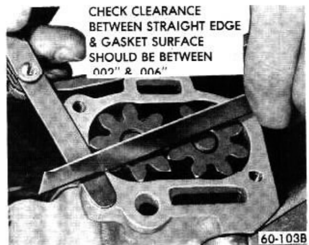
Figure 60-117 - Checking Oil Pump End Clearance
