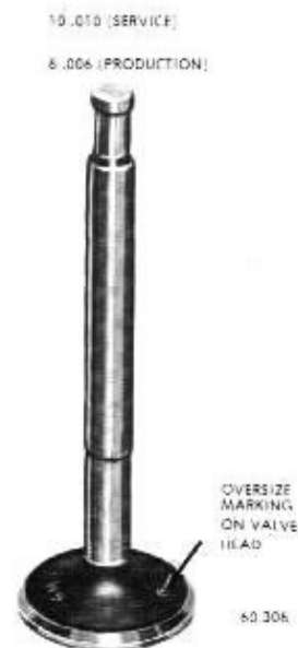
Figure 60-79 - Oversize Valve Identification
