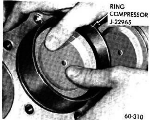
Figure 60-107 - Installing Piston with Ring Compressor Installed (350 Shown)
