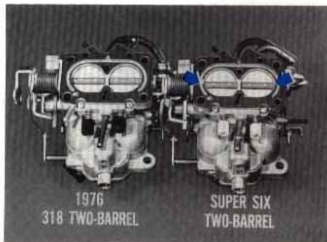
Fig. 4 — Notches provide source for vacuum signals
