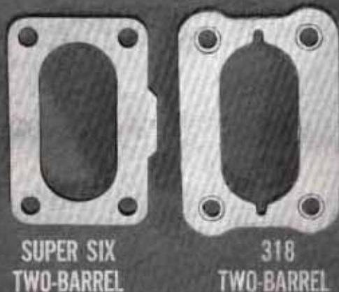
Fig. 5 — The Super Six "bathtub" design base gasket
