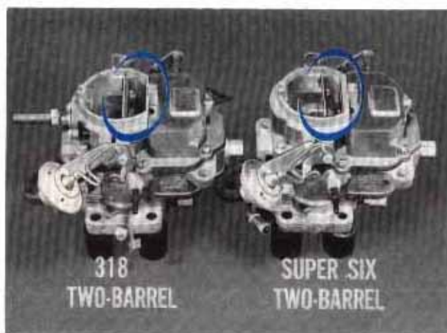
Fig. 7 — The Super Six air horn wall is thicker
