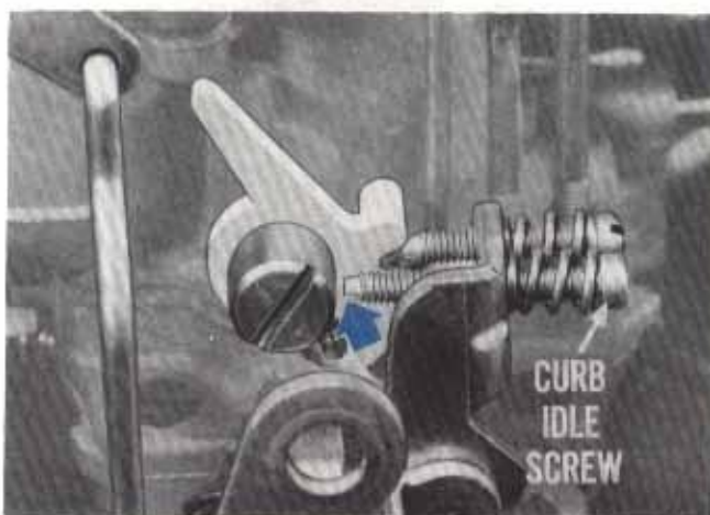
Fig. 21 — Throttle valves must be completely closed
