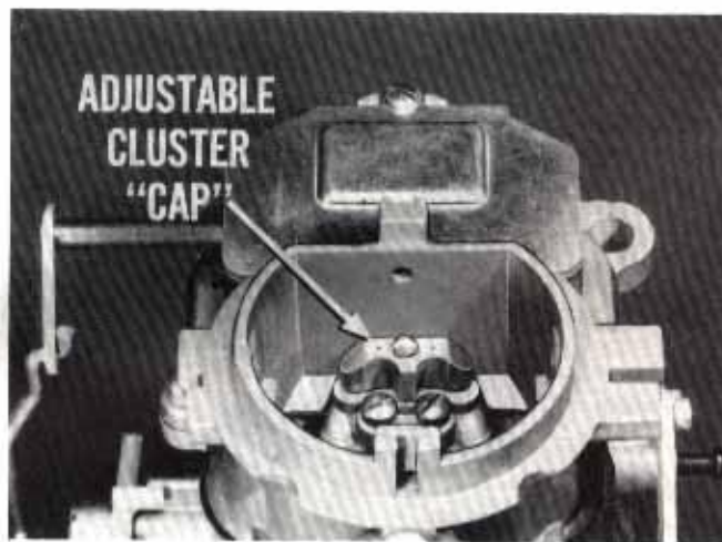
Fig. 34 — Manually adjusted high altitude compensator
