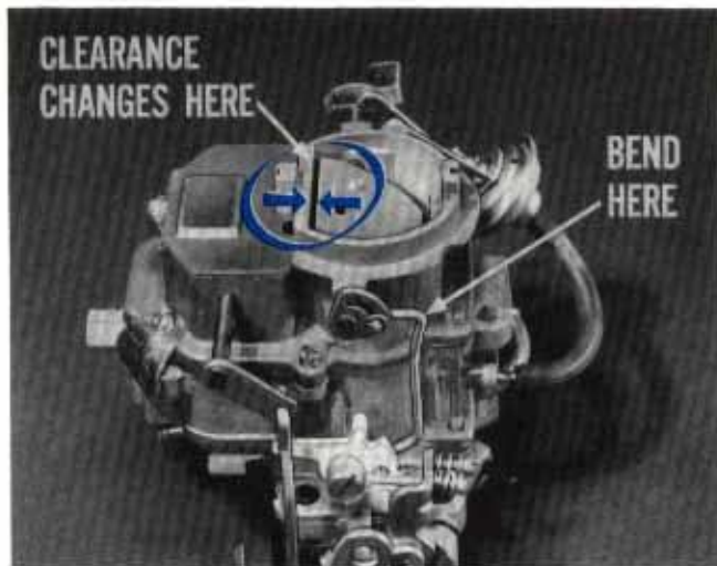
Fig. 15 — Bend carefully to change choke valve clearance
