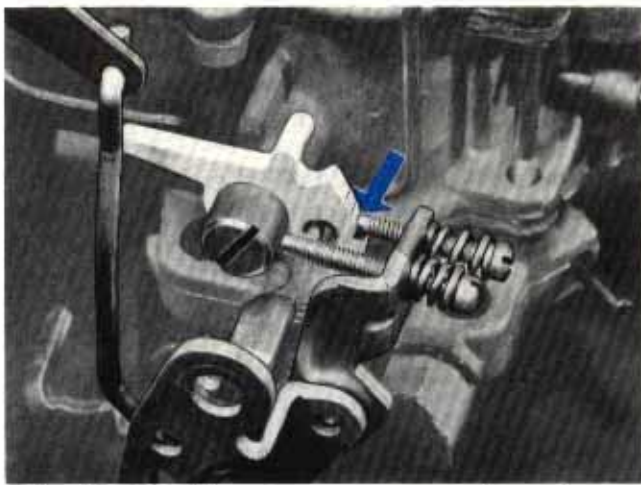
Fig. 13 — Fast idle screw rests on second step of cam
