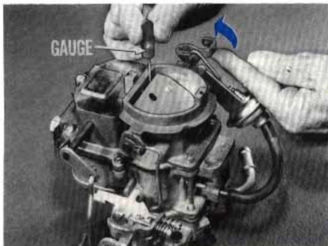
Fig. 14 — Checking fast idle cam position with gauge
