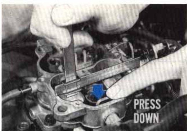
Fig. 29 — Be sure to press down on float pin retainer
