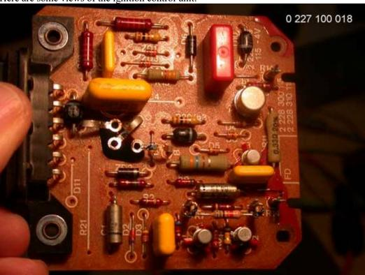
Here is R14 – clamped to the heat sink:
