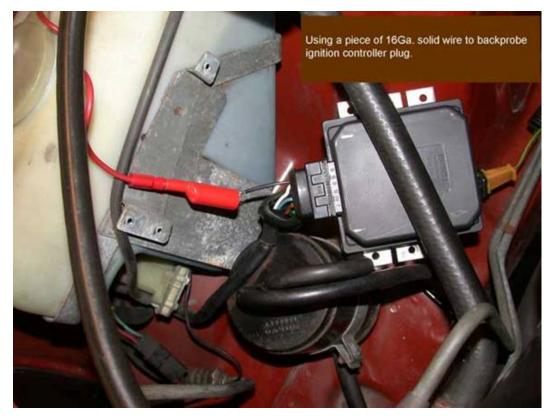
This approach to probing the circuit got me into trouble. The 16 Ga. wire is a perfect pin extractor. Make sure the tan not get released or the plug will push the terminal out of the socket housing.
