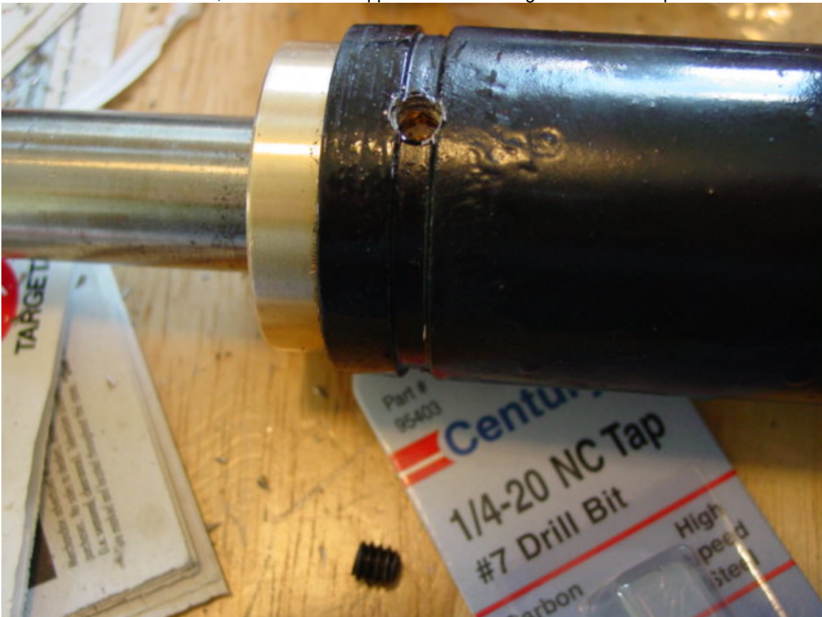
I choose to use set screws, and drilled and tapped the holes using a 1/4-20 NC Tap and #7 drill bit.
