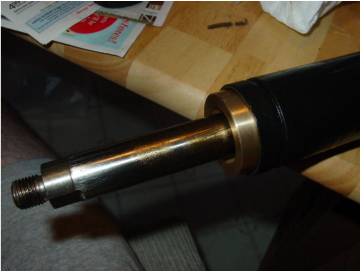
I choose to use set screws, and drilled and tapped the holes using a 1/4-20 NC Tap and #7 drill bit.
