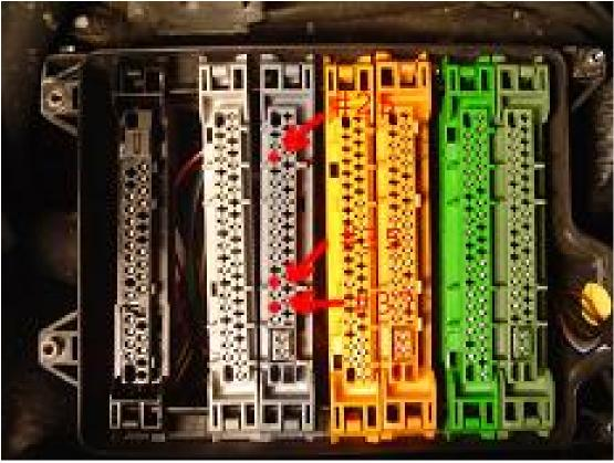
You cut the 3 wires. Then you mount 3 relays. One for each of the wires you should cut. Then you only have to mount the switch that turn on and of the relay inside the car.
