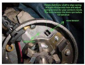
After complete reassembly of your distributor again make sure that the upper shaft returns to the idle position via spring tension. Adjust the spring tension adjustment arms so that the shaft returns to the idle position via spring tension if necessary. You can access the adjustment arms through the square access hole, adjust tension when the distributor is in the engine and you can check RPM to full advance with a dialback timing light. The shaft has to be still to make this adjustment.
