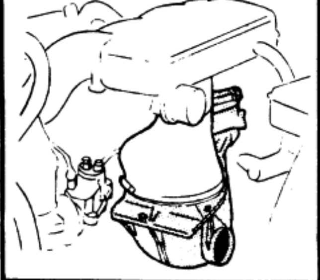
Air-fuel control unit
