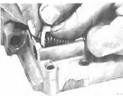
Place valve ball in position Compress spring and retainer together
