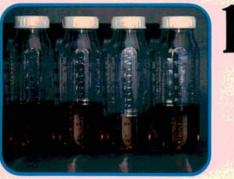
The most cost-effective tools for K-Jet injector volume tests are plain old baby bottles. Use one bottle per injector. Turn on the fuel pump, move the air flow sensor plate, and collect a few ounces of fuel. Line the bottles up on a level surface. The lowest fuel level pinpoints the leanest cylinder.
