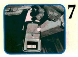
When the fuel pump fuse keeps blowing or the pump sounds draggy or noisy, check the pump's current draw. A typical K-Jet pump draws about 8 amps. Remember that the brown wire connected to the thicker-diameter terminal is the ground wire.
