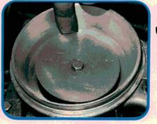
Checking injector flow/volume on a problem car? Remember to take three separate readings at three different sensor plate positions. Check it with the sensor plate barely open, with it halfway open, and with it wide open. At each of these plate positions, the injector's volumes should be equal.
