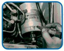
Most of the problems you encounter on K-Jet fuel systems are originally caused by damp and/or dirty fuel. You really can't change fuel filters too often on this system—but try convincing the customer of that! When you replace a filter, it can't hurt to log the mileage right on the filter can.
