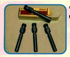
Would you replace just one bad spark plug instead of replacing the entire set? No? Then apply the same reasoning to injectors. Explain to customers that replacing just one injector-especially on highermileage engines-is false economy. Replacing all the injectors is cheap insurance.
