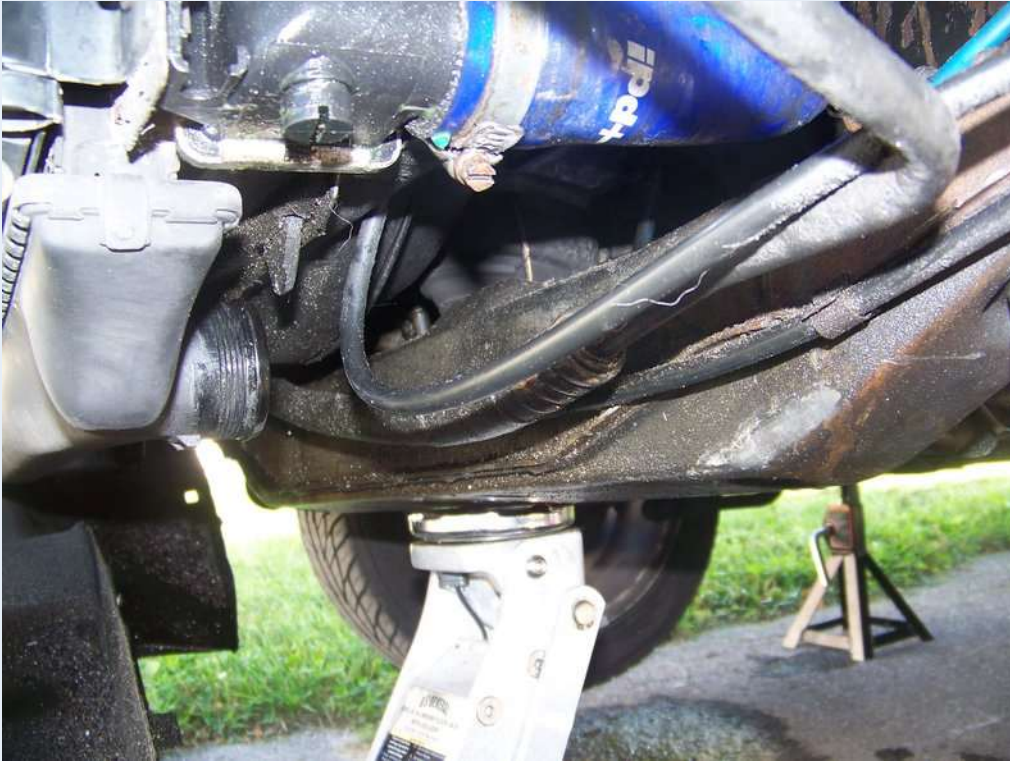
Lower Hose Released At Intercooler
