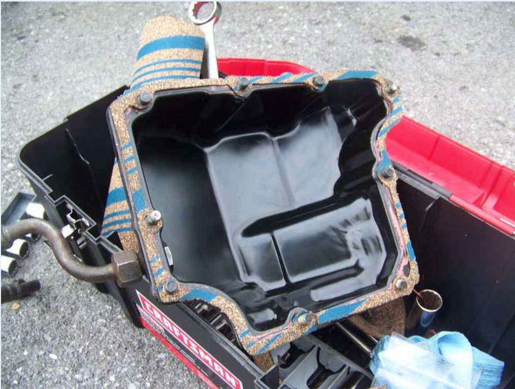
1st try at making a gasket.
